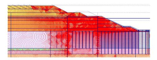
Figure 6 (b) Numerical Analysis by Plaxis, displacement vectors
