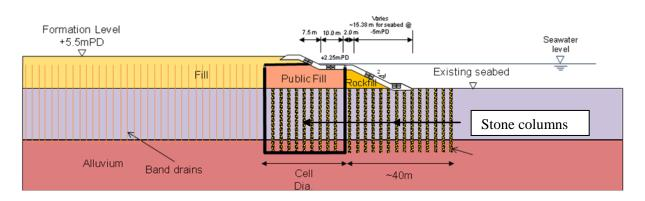
Figure 9 Undredged Seawall for HKBCF
