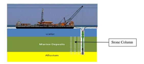
Figure 5 Stone Column as ground improvement technique
