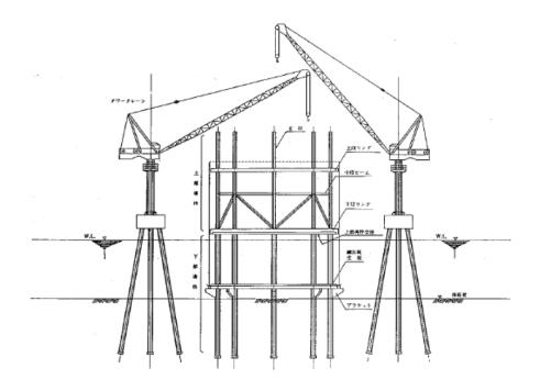
Figure 7 (a) A Schematic prefabrication yard
