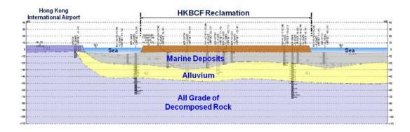
Figure 3 Cross sectional profile of geological stratification
