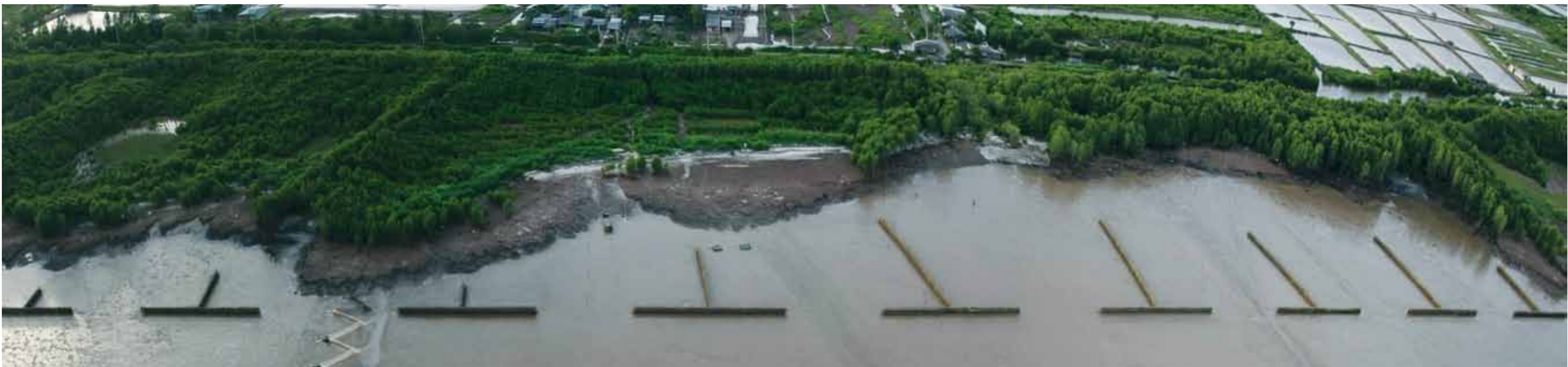
Figure 47: Second construction phase of T-shaped bamboo fences on the coast of Bac Lieu Province (Photo: Cong Ly and GE Wind)
