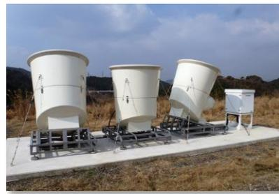
▲ Doppler SODAR system (Tri-monostatic)
