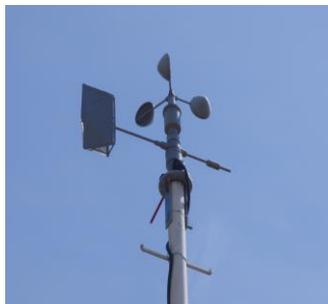
▲ Anemometer (Combined arrow feather and a three-cup anemometer)
