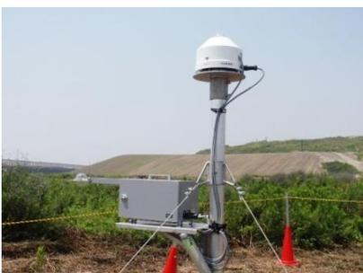
▲ Solar radiation meter and Net radiation meter
