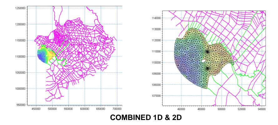
The 2D-hydraulic network set for the entire Bay of Rach Gia The network is divided into 5493 irregular triangular elements and 2864 computation points
